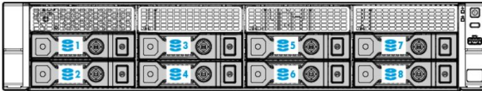
8-bay LFF hot-plug drive model
