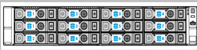
12-bay LFF hot-plug drive model
