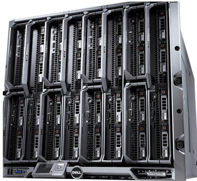
Figure 1. M1000e chassis front view
